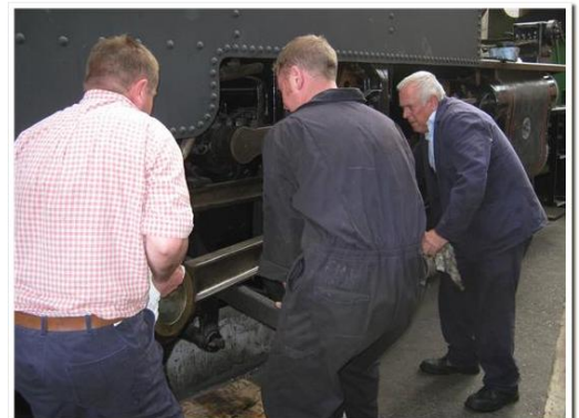
Andrew Summers, Steve Smart and Len Pullinger fitting one of the connecting rods to 41298 on 13th August
