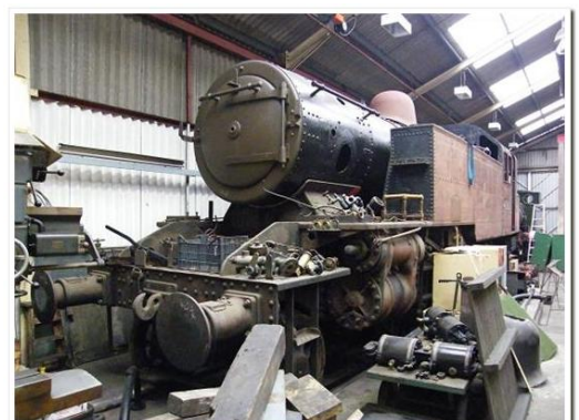
41313 - now with the correct boiler on the frames.
