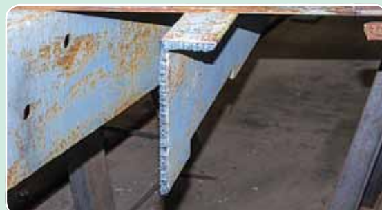
Folded diagonal section of SECR 6375's underframe cut out and ready to be prepared for welding.
