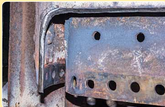
Firebox on Invincible showing accessibility to outer wrapper side plates with front and rear plates cut away and foundation ring removed. John Faulkner
