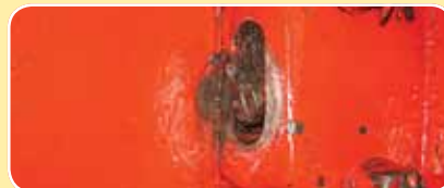
Failed leading front left-hand axlebox wedge pinch bolt on W24 Calbourne . Andrew Summers
