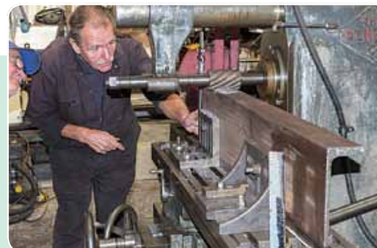
John Thorn setting up to machine the top face of one of the replacement sections for SECR 6375's underframe.
