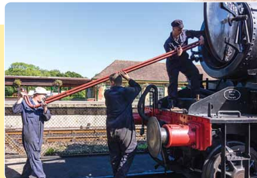
New superheater element being installed in 41298 and (right) completed installation. John Faulkner
