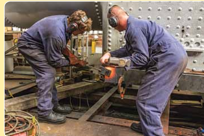
Forming a new outer wrapper side plate on Waggoner 's boiler. John Faulkner
