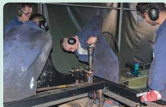
Alex Hull riveting one of the new bogie corner spring brackets into position on SECR 6375.
