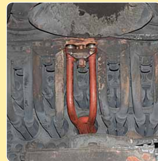
New superheater element being installed in 41298 and (right) completed installation. John Faulkner
