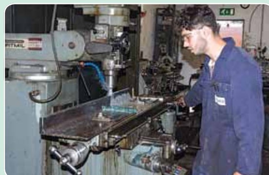
Callum Culver machining the side-face of one of the replacement sections for SECR 6375's underframe.
