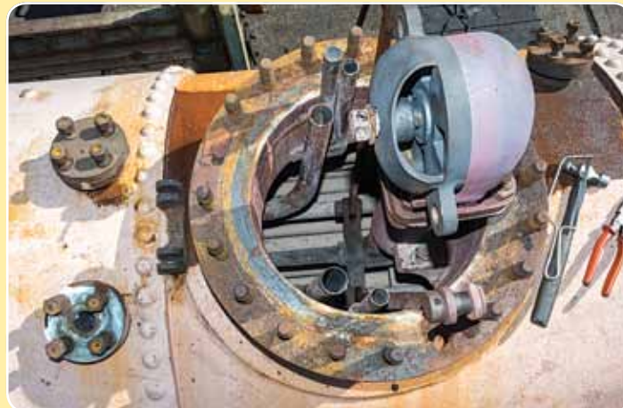
Boiler from W8 Freshwater with dome removed to allow for internal inspection and access to blank off the regulator head for the hydraulic test. John Faulkner
