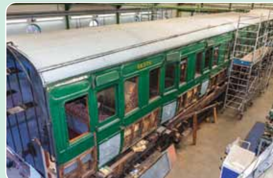
The south side of 6375's body with all of the lower panels removed.
