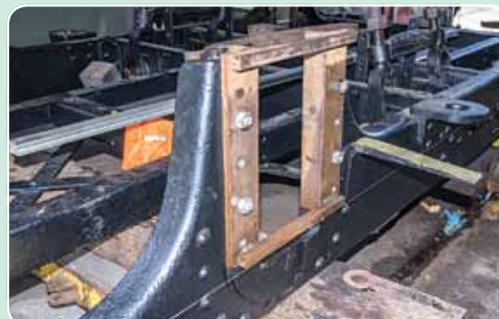
New horns ready for riveting onto the bogie of SECR 6375.
