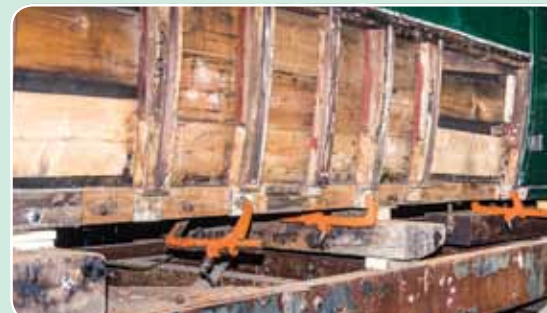
Section of SECR 6375's body with rotten timber cut out and awaiting new timber to be fitted.
