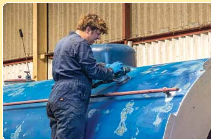
Waggoner 's saddle tank being prepared for priming. John Faulkner
