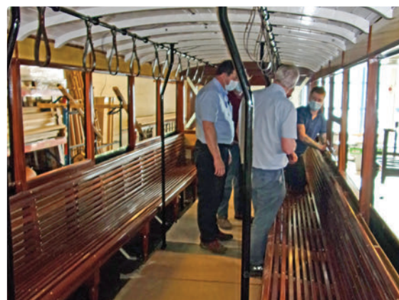
Car 2: Detail includes completed seats, roof support poles and hanging poles with leather straps.
