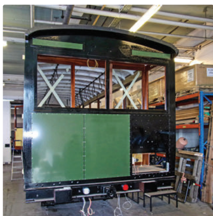
Car 2: 'Temporary' rear glazing on the verandah end. It's almost too good to take off!
