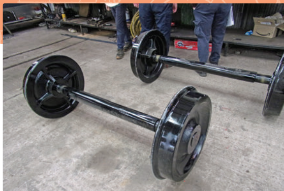
Completed wheel sets for Car 10 All photos by Terry Hastings
