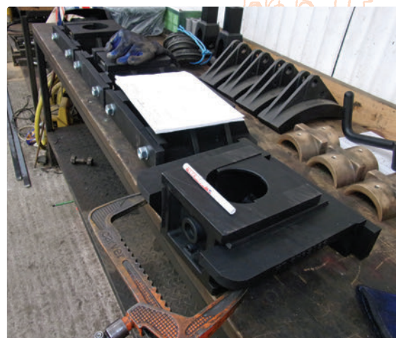
Car 10: Sundry items including brake parts and wheel bearings on the bench for inspection.
